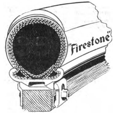
Fig. 1—Firestone demountable rims for Fords
